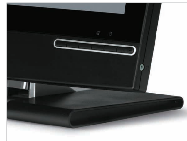
DVI input, built-in speakers and easy access headphone jack for multimedia and interactive applications
