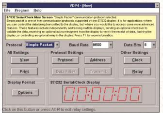
For advanced display applications, nothing beats Vorne Display-Pro® software for providing simple yet powerful setup of your 87 series display. Over one hundred programmable parameters are at your fingertips, in a point and click environment that is consistent throughout the 87 series family of products. Addresses, ID tags, trigger points, presets, scale factors, input characteristics, display ranges, and much more are all easily modified. And of course the software is yours free of charge.
