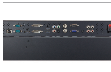
Mutiple video inputs (VGA, DVI, HDMI, BNC, S-Video, DisplayPort and Component) allow for effortless system integration
